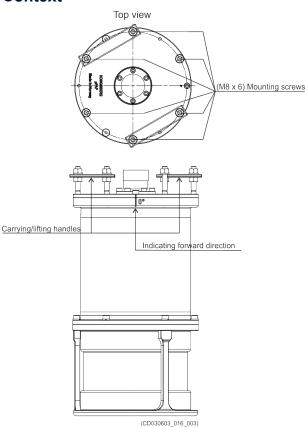
The transducer is mounted on the ship's arrangement for the transducer. This may be on a pole lowered through a moon pool or a hull unit.
